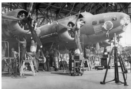
Legendary B-17 “Suzy-Q” undergoing depot maintenance at Hill Field.
