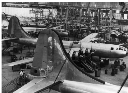
Ogden Air Materiel Area B-29 maintenance line, 1950. Some B-29s would be modified with air-to-air refueling capability.
