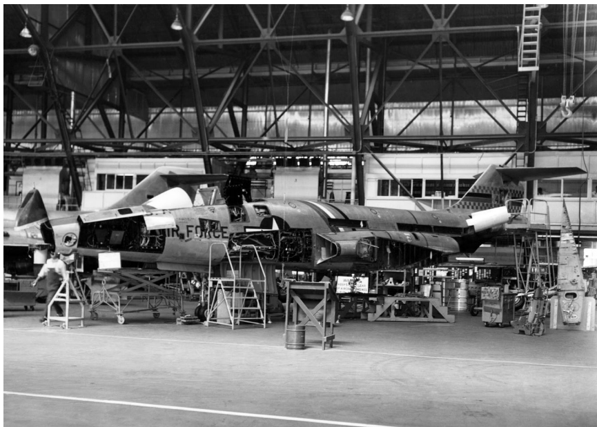
This June 1959 photograph shows an RF-101 jet reconnaissance aircraft under repair in the depot maintenance line, Hill Air Force Base, Utah.
