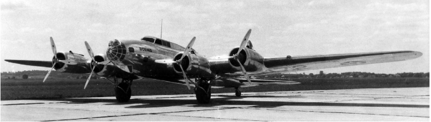
Boeing Model 299, prototype of the B-17 Flying Fortress. It could fly 250 mph at 14,000 feet and operate at a max ceiling of 30,000 feet.
